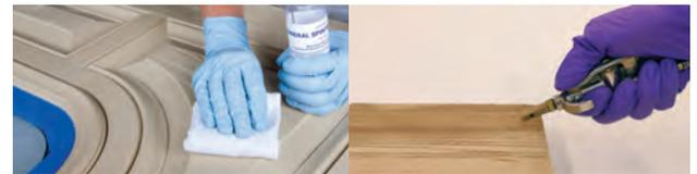
Prior to staining, be sure to clean and prepare surfaces. Use a cleaning rag dampened with mineral spirits to wipe the entire surface, removing all contaminants.
