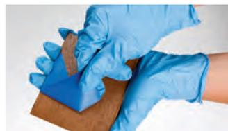
To determine if the stain is dry enough for applying topcoat, stain the unstained fiberglass test sample. Allow to dry for at least 6 hours before testing for dryness and applying topcoat.
